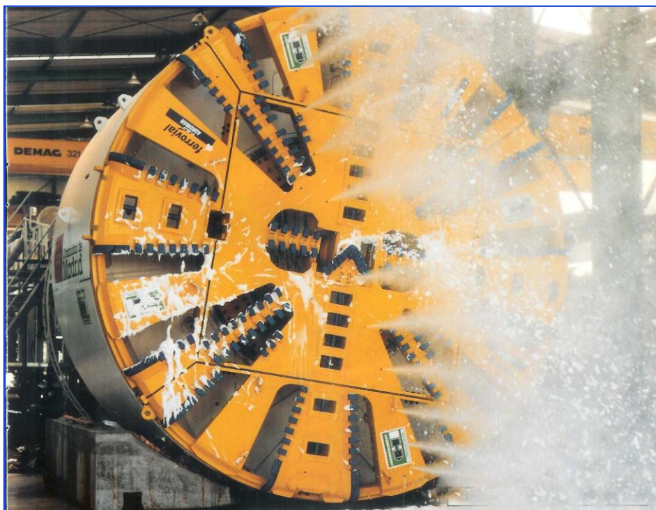
Typical discharge of soil conditioner from several ports at the cutterhead.
