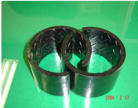
Photo 11 Joint of the piles
