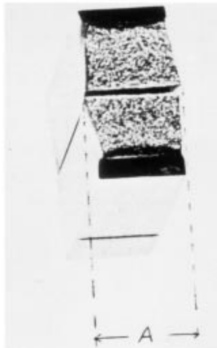
FIG. 15 Halves of Broken Charpy V-Notch Impact Specimen Joined for the Measurement of Lateral Expansion, Dimension A
